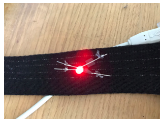
Figure 12. System works with conductive wires
