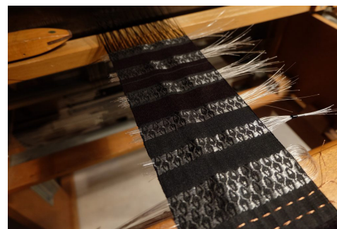
Figure 9. EL wires woven with thread IMG from Audrey Briot [Briot, 2015]
